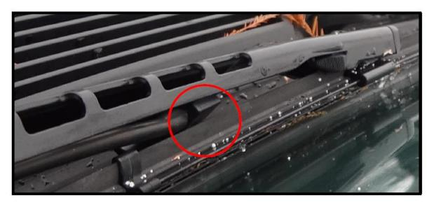
The original blade is 16.5mm high (.65 in.), measured from the bottom of the squeegee to the tip of the spoiler. The OE spoiler is located off-center to the rear of the wiper blade. Some aftermarket blades are of varying height and many have the spoiler down the middle of the blade. The different height and location vs. the OE blade may allow the spoiler to press against the washer nozzle affecting wipe quality.
